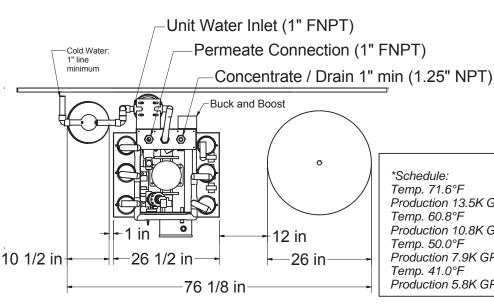
\*Schedule: Temp. 71.6°F Production 13.5K GPD Temp. 60.8°F Production 10.8K GPD Temp. 50.0°F Production 7.9K GPD Temp. 41.0°F Production 5.8K GPD
