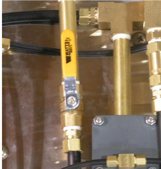
Figure 3-5. Filter Change Shut Off Valve
