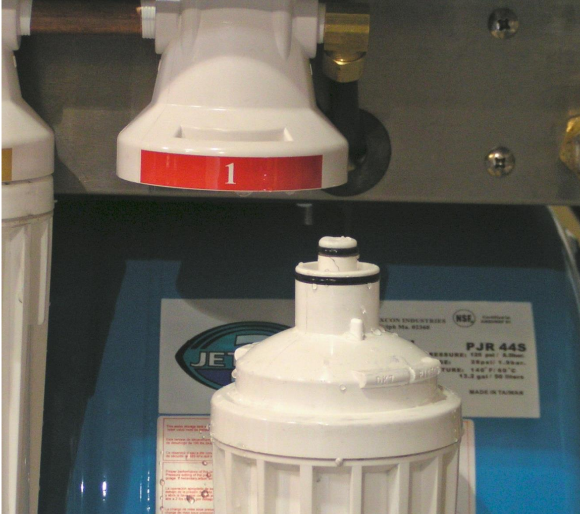
Figure 4-8. Install Pre-Treatment Filter Cartridge One (1)
